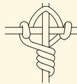
The Tornado Titan joint is an innovative non-slip knot incorporating a continual vertical stay wire. It has exceptional impact resistance making it ideal for high pressure applications.
