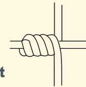
Traditional cost effective joint. Enables the netting to be turned out or cranked for use in special applications.
